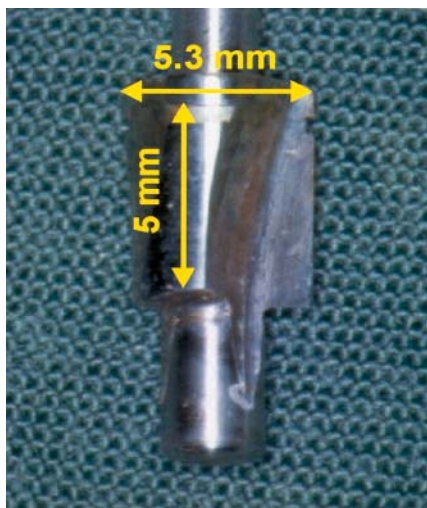
Fig. 1. The step drill used to prepare the defects at the test sites. The diameter of the upper, cutting part of the drill was 5.3 mm.
