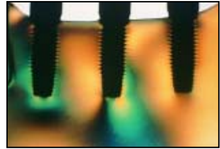
Fig 4b (right) Stresses produced by 89-N vertical load upon anterior implant: staggered configuration model.
