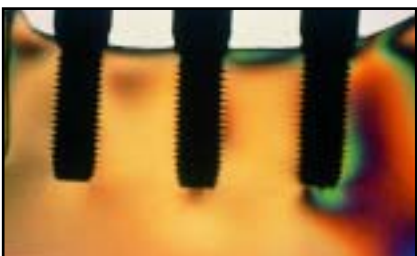
Fig 8a (left) Stresses produced by 89-N posteriorly directed load upon middle implant: straight configuration model.
