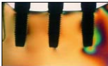
Fig 8b (right) Stresses produced by 89-N posteriorly directed load upon middle implant: staggered configuration model.
