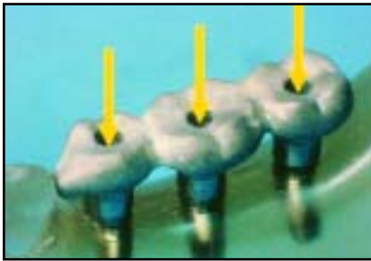
Fig 3a (left) Locations of load point applications: Vertical load is applied separately to each location.
